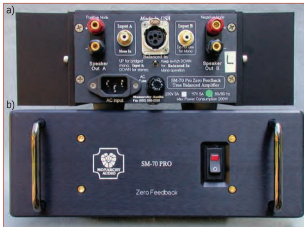
Photo 4: A pair of Monarchy SM-70 Pro power amplifiers are pictured with the rear panel (a) showing the unbalanced RCA connectors for stereo connections and a single XLR connector for fully-balanced monaural operation.
