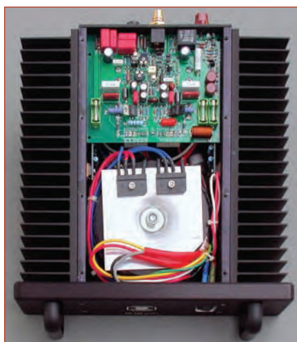
Photo 3: This is an inside view of the SE-100 MK2 amplifier. The new MOSFET output PC boards are mounted on the heatsinks, under the main PC board. The hefty, 450-VA toroidal power transformer and Shindengen low-noise, soft-recovery rectifier bridges are in the front portion of the amplifier.
